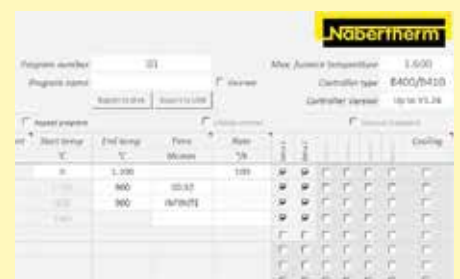
Process input via the NTEdit software (freeware) for MS Windows™
