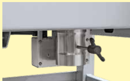
Semi-automatic air inlet flap for residual drying in chamber kilns up to 300 liters
