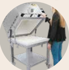
Ergonomic charging height of 860 mm
