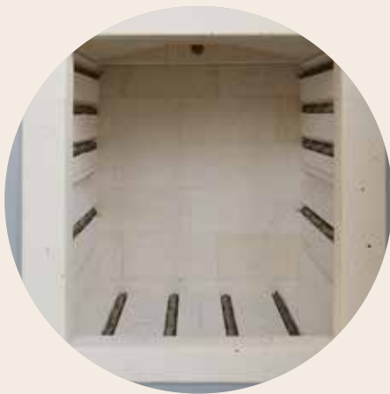
Three-sided heating with elements protected in grooves
